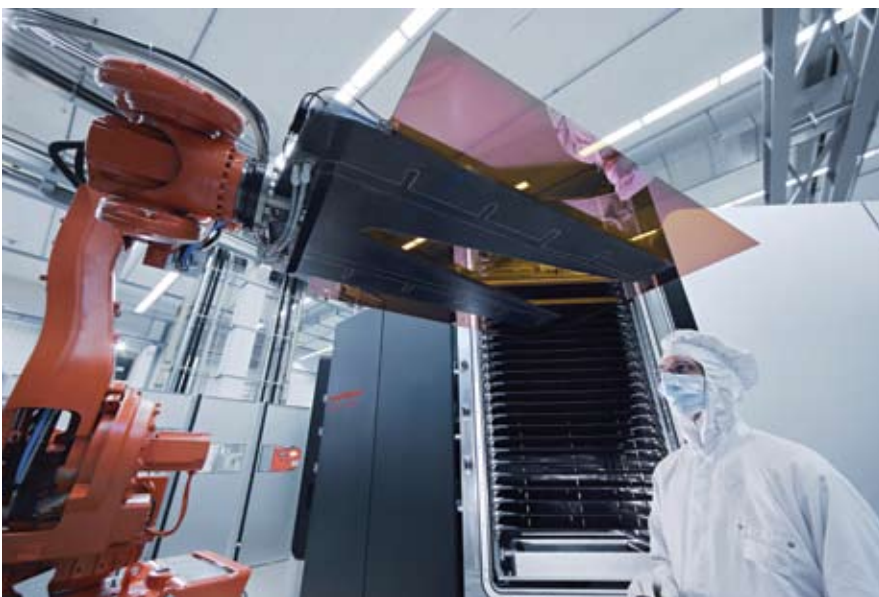
The KAI 1200 PECVD system from Oerlikon Solar is depositing the complex absorber layer on over 650 glasses of 1.4 m 2 per day
